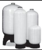
TAW FRP vessels are high pressure water filters specially designed for water treatment applications. They are especially suitable for water softeners and pre-treatment filtration for reverse osmosis plants where removal of suspended solids is essential. They are made from a combination of fibre reinforced with plastic making them robust and able to with stand pressures of upto 8bar and filtration velocity of 25m/sec/m2
