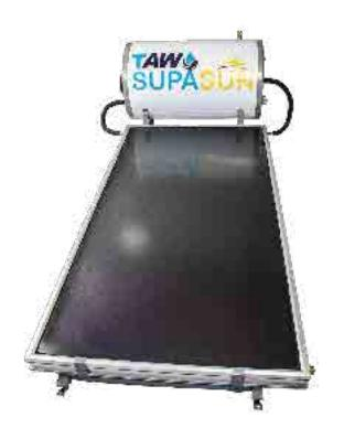
TAW Thermo-siphon solar water heaters are high efficiency low maintanance systems that are environmentally friendly and the most economic way to get hot water from the sun. The system uses natural water circulation to heat up the water and doesn't require a pump or contol unit. It includes solar collectors, storage tank and durable mounting sets.
